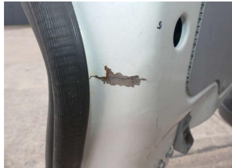
Hecktür links gerissen
